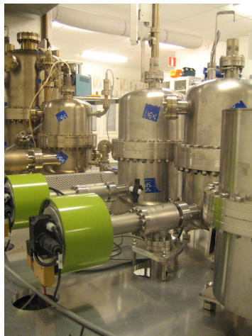
SP's reference equipment for vacuum metrology (static expansion) transferred from NPL (UK)
